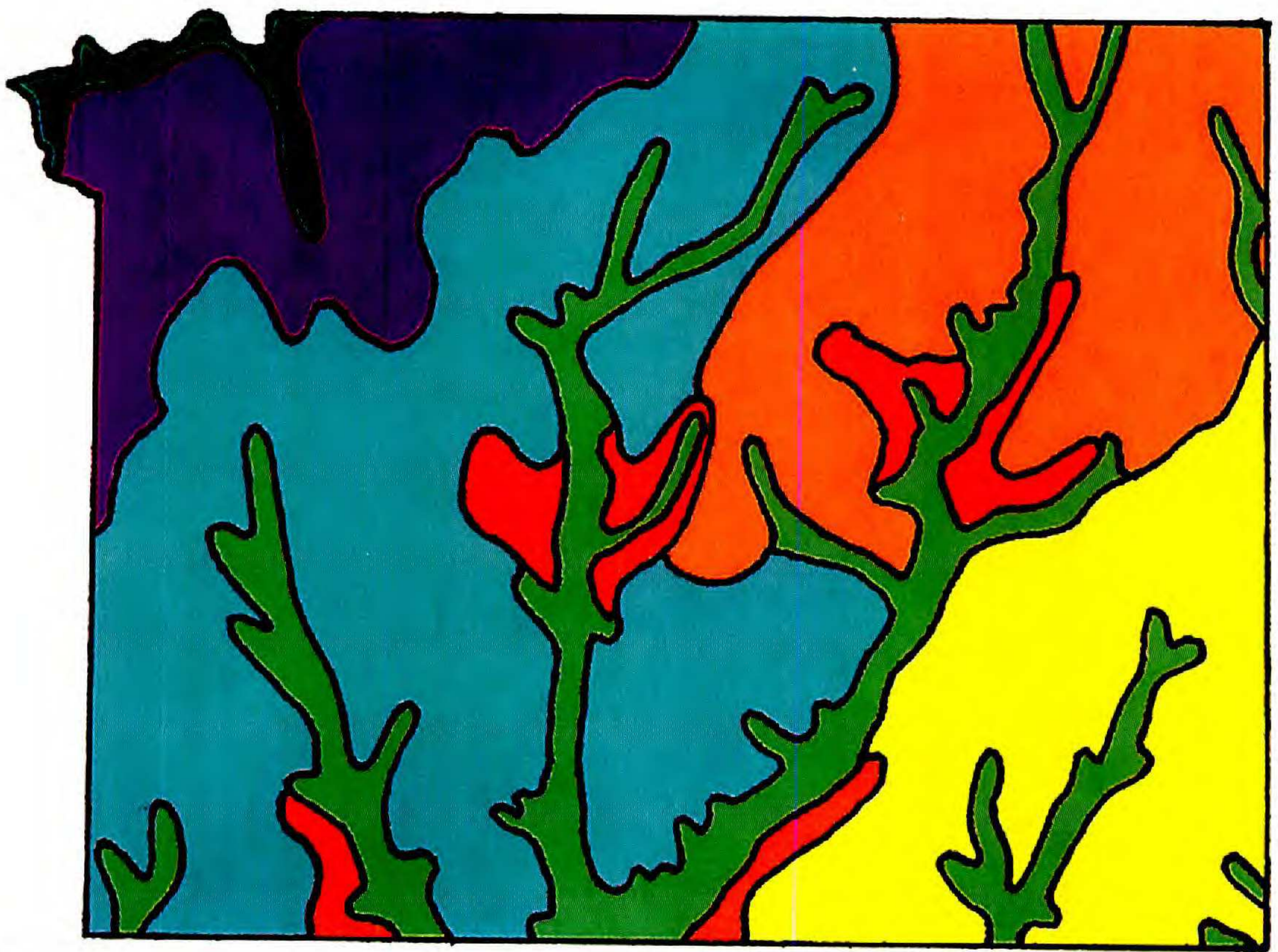
FIG. 2. Soil map of Amite County, Mississippi (adapted from Milbrandt, 1976). The Gillsburg-Ariel-Peoria association (flood plain) is in light green, Collings-Bude (flood plain) in dark green, Ora-Smithdale-Providence (upland coastal plain) in yellow, Providence-Bude in orange, Providence-Ruston (shallow loess) in blue, Saffell-Smithdale-Providence (often gravelly) in red, and Smithdale-Susquehanna (loam over clayey subsoil) in magenta.
